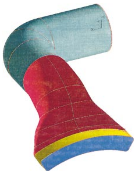
Fig. 12 Geometry of 90-deg elbow and transition piece downstream of MS3002J combustor
